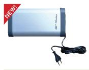
The DC10 can be used in combination with S3/S4 and almost any 220 VAC power source to form a power-ful continuous power supply (CPS) system. It provides a stable 12VDC output, straight to the aplication, or to the S3/S4. The unit is capable of handling a maximum load of 10A. In areas with bad electricity grid a CPS provides the comfort and security of never failing lamps and applications.
